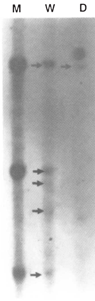
FIG. 1 Hybridization of probe 29C1 for the locus DXYS14 to Pst I-digested DNA from deceased mother (M), blood speck from defendant's watch (W) and deceased daughter (D), performed by Lifecodes in New York v. Castro . Although the autoradiogram shows three bands in lane M, five bands in lane W and one band in lane D, Lifecodes recorded three bands in identical positions in all three lanes. The autoradiogram is an overnight exposure; no further exposures or hybridizations involving this probe were performed.
