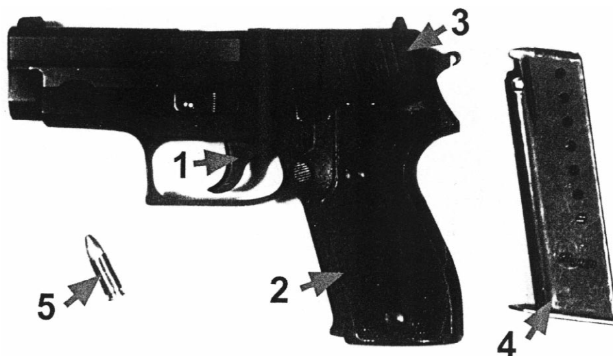
Fig. 1. Five areas of a pistol which were wiped with glass fleece to recover DNA traces: (1) trigger cock; (2) grip; (3) hammer; (4) magazine; (5) cartridge.
